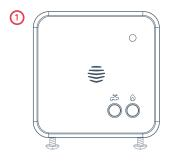
Loosen the screws on the underside of the receiver and remove the backplate by pulling the bottom of it away from the front panel.
